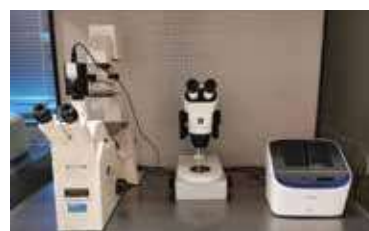
Fig. 2: Dissection hood containing a stereo microscope, Zeiss imaging system and the Countess III automated cell counter.
