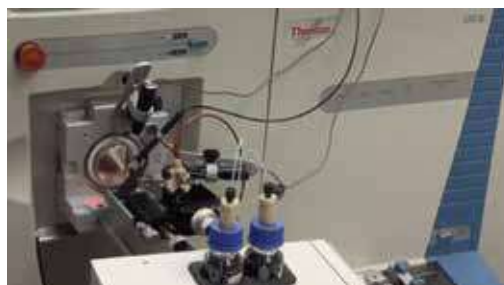
ProFI is equipped with an LTQ Orbitrap XL – ETD mass Spectrometer coupled to a nLC system with auto-sampler.
